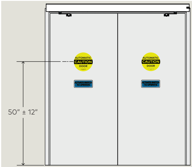
Fig. 8.6.3 Push/Pull, push to operate
