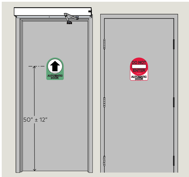
Fig. 8.3.1 One decal, one way traffic Approach Non-approach
